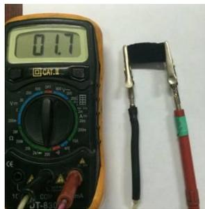
Figure 8 – Measurement of the resistance of fiberglass with CNT
