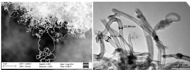
Fig. 2 SEM and TEM images of carbon nanotubes grown on glass-cloth with Co<sub>3</sub>O<sub>4</sub> (5 wt. %)
