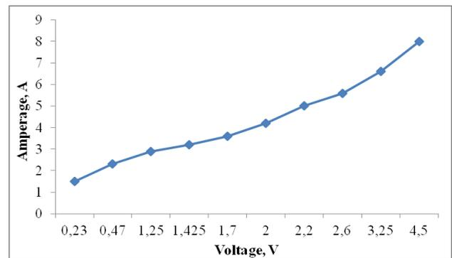
Fig. 4 Current-voltage characteristics of the sample of CNT@glass-cloth
