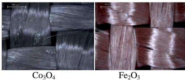
Fig. 1 Optical microscope photographs of glass-cloth with Co<sub>3</sub>O<sub>4</sub> and Fe<sub>2</sub>O<sub>3</sub>
