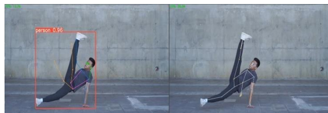
Pic 1: Performance Comparison: MediaPipe (Lite) vs. YOLOv8 (Extra Large) in Break Dance Scenario
