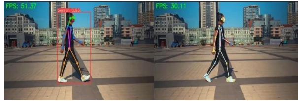
Pic 2: Performance Comparison: MediaPipe (Lite) vs. YOLOv8 (Nano) in Walking Detection Scenario
