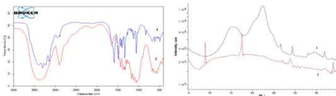
Fig.1. FTIR spectra and X-Ray diffractograms of cellulose (1) and cellulose nanofibers (2)
