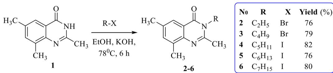
Reactions were carried out by boiling a mixture of reagents - **1**:R-X:KOH - 1:1.2:2 at the 78°C for 6 hours, and 2,6,8-trimethyl-3-alkylquinazolin-4(3H)-ones (**2-6**) were synthesized in good yields (76-82%).
