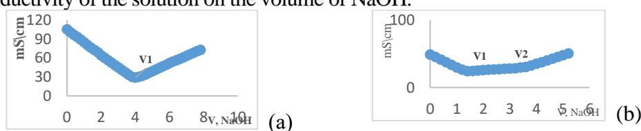
Fig.1. Conductometric titration curve of a blank solution of 0.1 N HCl and 0.5 M NaOH (a) and CH solution (b)
