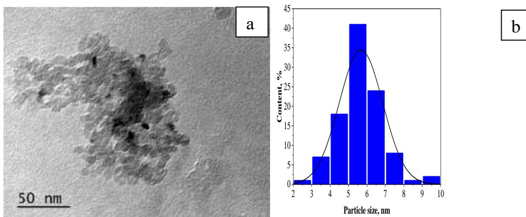
Fig. 1. -. (a) TEM image of BN nanoparticles; b – size distribution of nanoparticles
