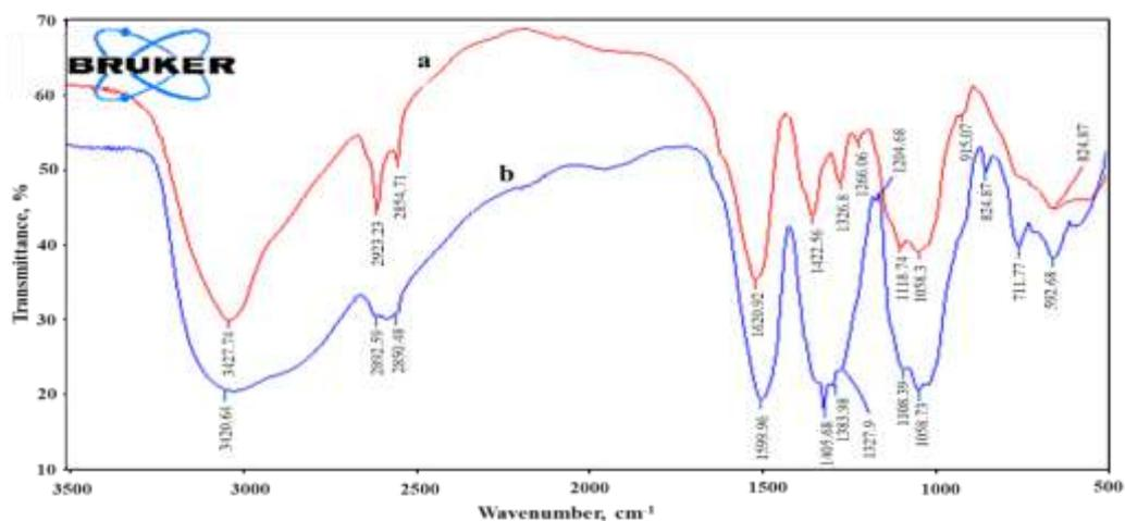
Fig. 1. Purified Na-CMC (a) and  $\text{Ag}^+\text{CMC}^-$ , (b) films FTIR-spectrum results
