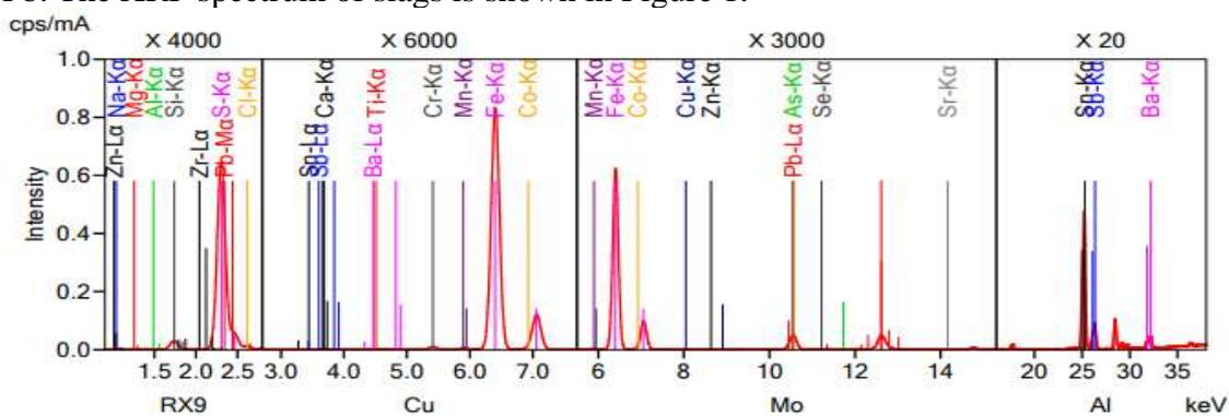
Figure 1. XRF spectrum of soda slag.
