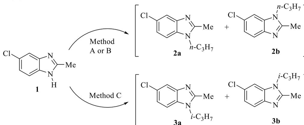
Method A:  $1:C_3H_7Cl:K_2CO_3$  - 1:1,5:1, acetone, 56<sup>0</sup>C, 10 h (Yield: **2a+2b**, 58%);
