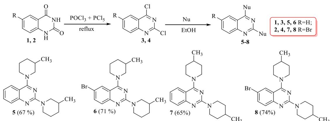
Experiments were conducted by heating mixture of 2,4-dichloroquinazolines (**3,4**) and piperidines in a 1:3 ratio in an absolute ethanol ( $80^\circ\text{C}$ ) for 6 hours, and corresponding compounds **5-8** were synthesized. The structure of the obtained substances was confirmed based on the results of IR,  $^1\text{H}$  and  $^{13}\text{C}$  NMR-spectra.
