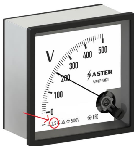
Figure 132 - Voltmeter with accuracy class 1,5
