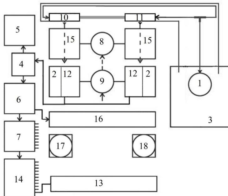
1 - submersible pump; 2 - Green panel; 3 - bath; 4 - Battery charge controller; 5 - Battery; 6 - Power supply unit; 7 - Automation unit; 8 - Motor plate reducer; 9 - Motor reducer of panels; 10,11 - Wipers with spray panels and plates; 12 - Solar panel; 13 - LED Illuminator; 14 - Switchgear; 15 - Acrylic plates; 16 - High voltage electrode; 17,18 - Fan;
