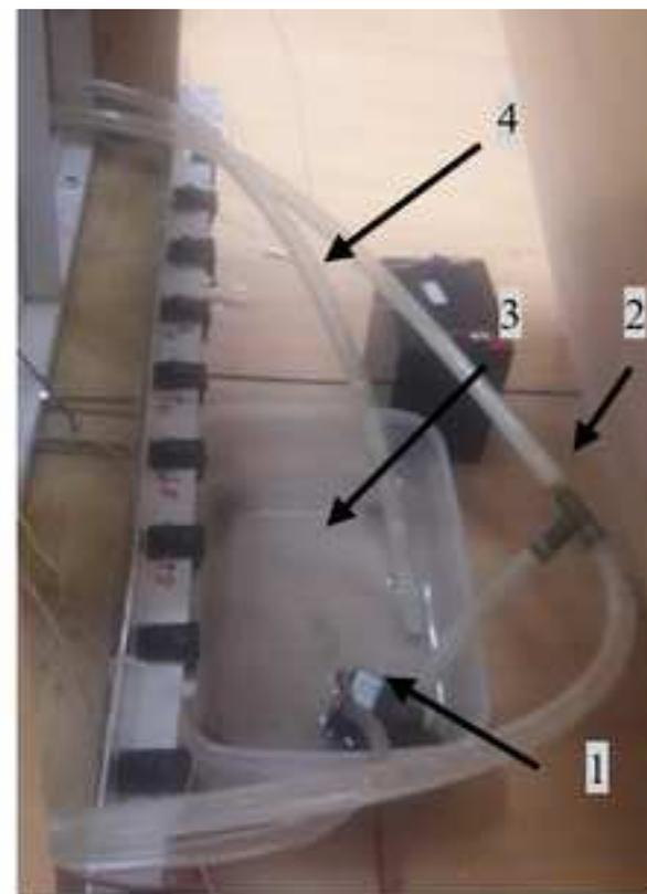
1 - submersible pump; 2 - tee; 3 - bath; 4 - pipe to return water; 5 - enter of water to an acrylic tube; 6 - return water collection funnel
