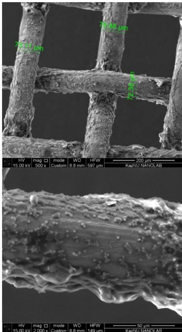
Fig. 2 SEM images of the surface of membranes based on a stainless steel mesh 200 coated with PDDA/SiO<sub>2</sub>
