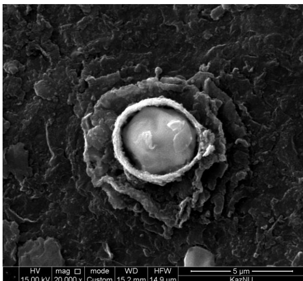
Fig. 2. Single images of the dust “projectile” appearing during the arc discharge and the destruction of the surface with a dust.
