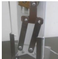
Fig. 9. Prototype of the new crank press.
