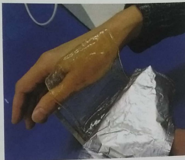
Figure 1. The photo of synthesized hydrogel wound dressings based on polyvinylpyrrolidone, agar, chitosan and polyethylene glycol as a plasticizing agent.
