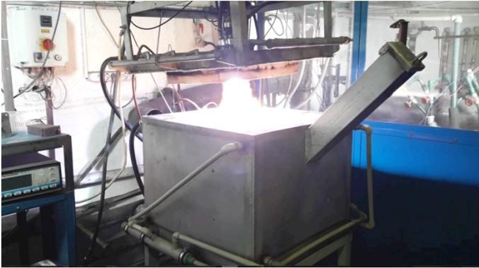
Figure 6. Photo of the plasma torch in action with lifted lid of the reactor.
