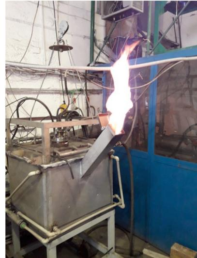
Figure 7. Photo of the combustible gas control flame from the pipe for supplying of briquetted FW.
