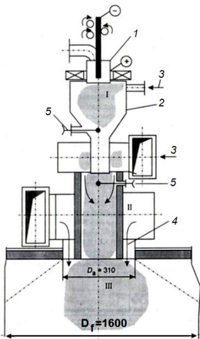
Figure 1. Layout drawing of plasma-fuel system and experimental furnace: 1 - plasmatron; 2 - chamber of electro-thermochemical preparation of fuel; 3 - pulverised coal; 4 - secondary air; 5 - slot for measuring; I - zone of air/coal mixture interaction with plasma flame and HRF forming; II - zone of HRF interaction with the main air/coal mixture; III - zone of the fuel self-ignition.
