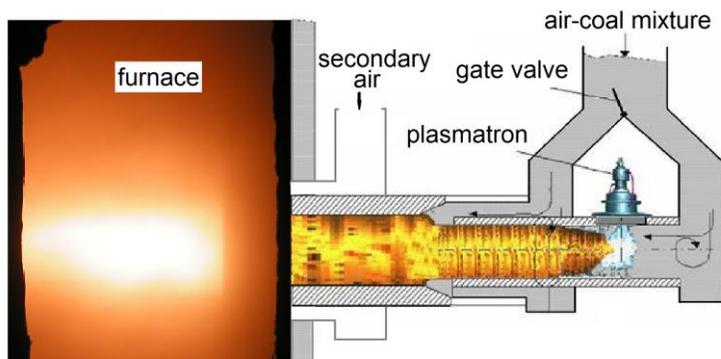
Figure 8. Sketch of the PFS for replacement of the traditional burners of the boiler BKZ-75.
