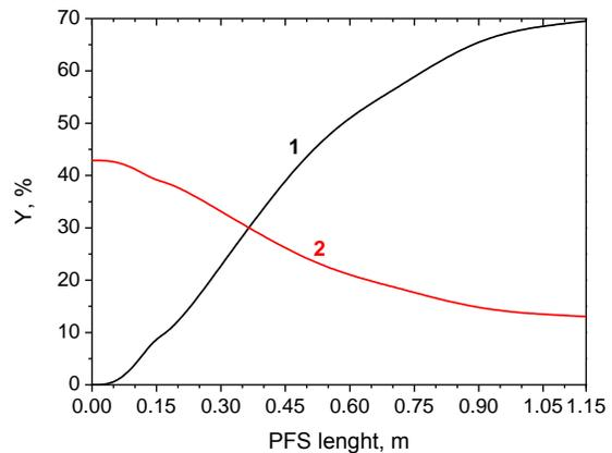
Figure 4. Gasification degree (1) and carbon concentration (2) in coke residue along the PFS.
