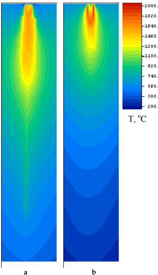
**Figure 5. Temperature fields along the furnace height in the central section for conventional (a) and plasma supported (b) regimes.**
