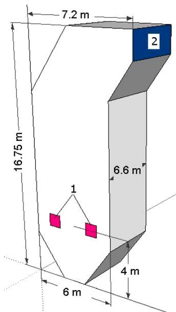
**Figure 7. Layout of the furnace of BKZ-75 power boiler: 1-burner throat; 2-section of the swiveling chamber of the boiler.**
