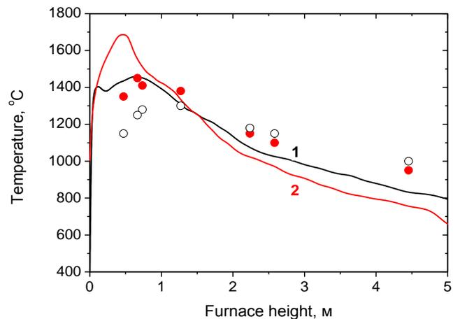
**Figure 6. Furnace height distribution of the combustion products maximal temperature: 1 - conventional incineration of coal; 2 - incineration of coal in the furnace with PFS; ●, ○ - experimental data on coal incineration in the furnace with PFS and without PFS correspondingly.**
