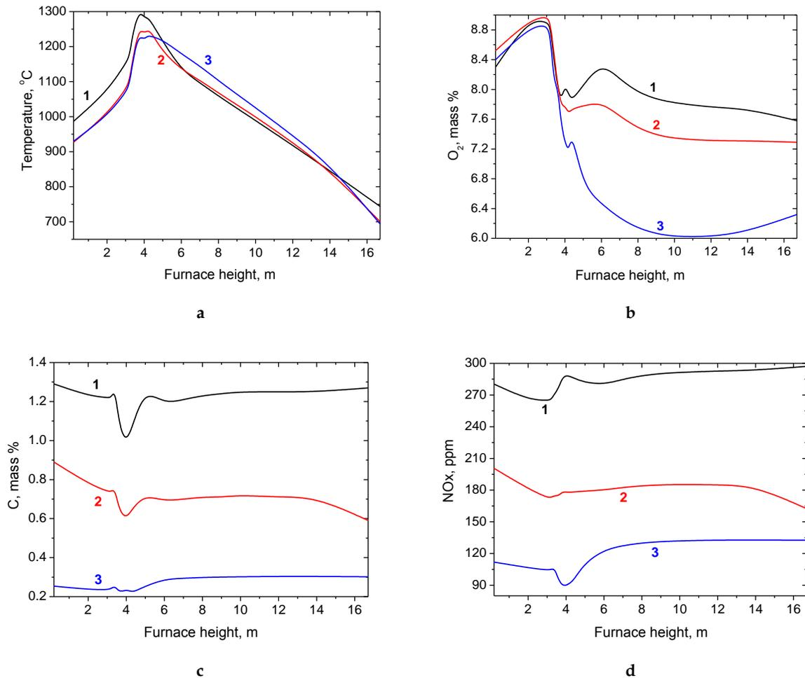
Figure 10. Furnace height distribution of mass average temperature (a), oxygen (b), carbon (c) and NOx (d) mean concentrations: 1-standard operational regime; 2-plasma operational regime with two PFS; 3-plasma operational regime with four PFS.
