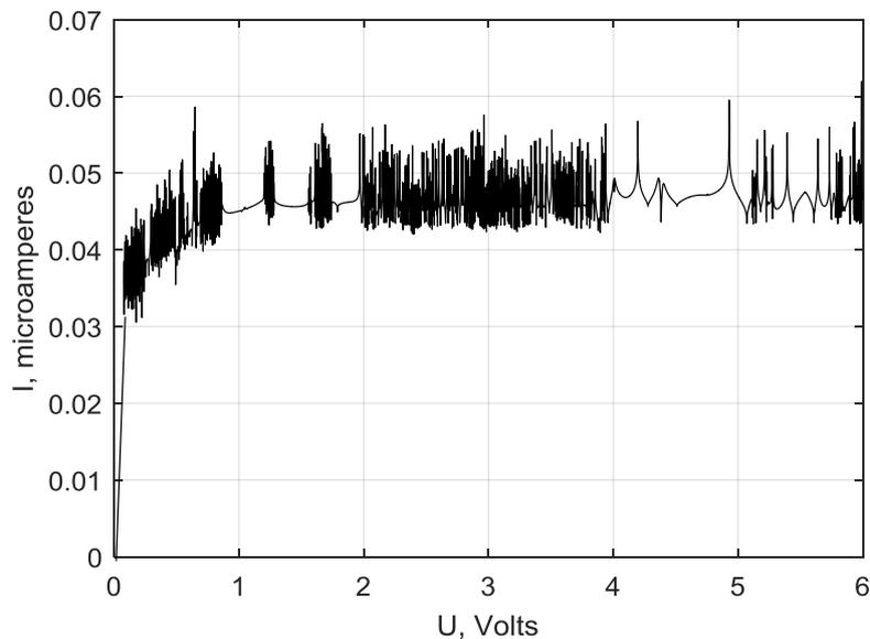
**Fig. 1.** Current-voltage characteristic of quantum nanowire.
