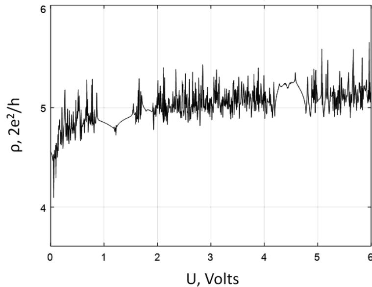
**Fig. 2.** Dependence of conductivity of quantum nanowire on external voltage.
