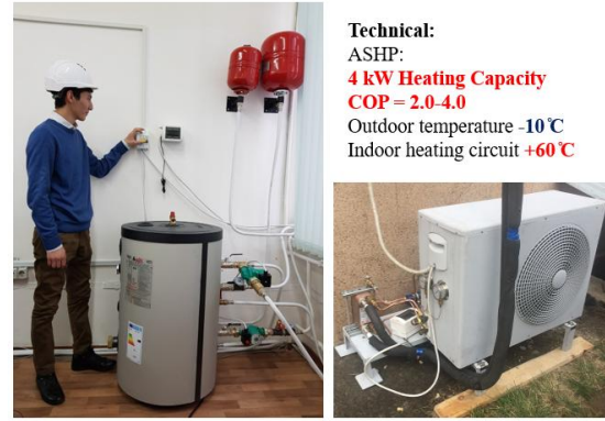
Fig. 3. Experimental setup of air source heat pump
