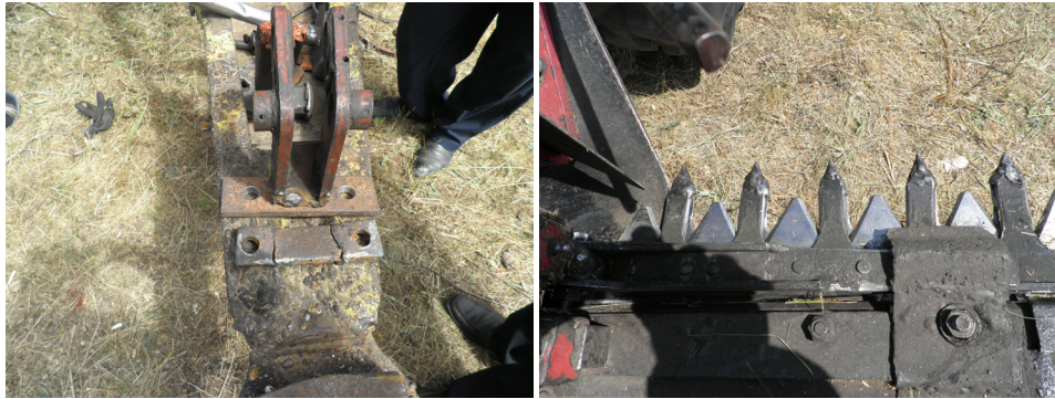
Fig. 1. "Holland" 55–56 (FD-2,10) typical failures while operating on the haylands littered by stones
