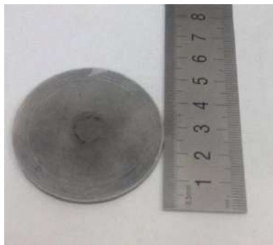
Figure 1 - Solid oxide target for pulsed laser deposition
