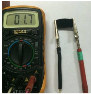
Figure 8 – Measurement of the resistance of fiberglass with CNT
