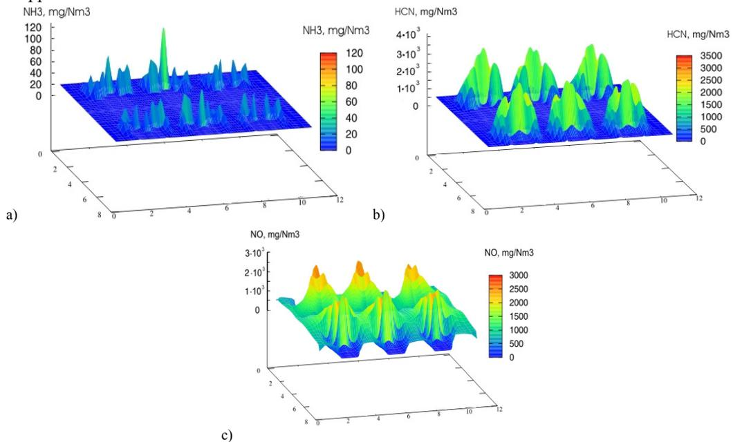
Fig. 2. Distribution of the concentration (a) - ammonia  $\text{NH}_3$ ; (b) -  $\text{HCN}$ ; (c) -  $\text{NO}$  nitrogen monoxide in the combustion chamber of the boiler SB-39 in the field of lower level of the burners
