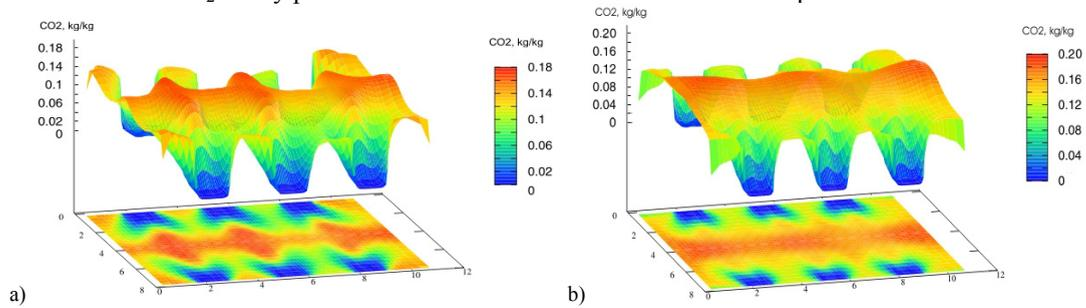
Fig. 1. 3D concentration distribution of  $\text{CO}_2$  in the combustion chamber of the SB-39 in the field of burner (a) - lower level; (b) - the top-level
