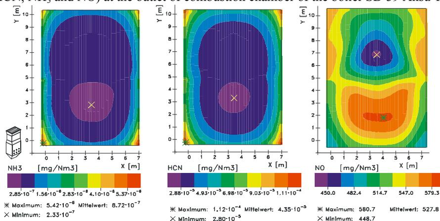
Fig. 3. Distribution of the concentration of nitrogen compounds at the outlet of combustion chamber of SB-39 of Aksu TPP
