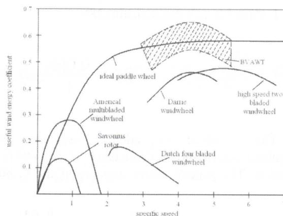
**Figure 4** – Dependences of operating ratio of wind power  $\chi$  for various types and designs wind turbine from degree of their rapidity  $c$ .
