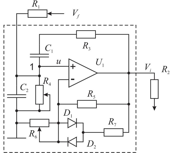
Fig. 2. Wien bridge oscillator. Here  $V_i$  is the output voltage of the  $i$ -th oscillator,  $V_f$  is the output voltage of the global feedback loop.
