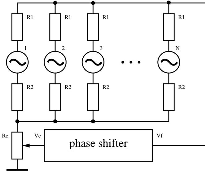
Fig. 1. Scheme of the globally coupled system. Individual generators are shown here by one symbol, their detailed scheme is given in Fig. 2, whereas the scheme of the phase-shifting unit is given in Fig. 3.
