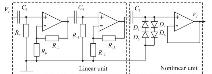
Fig. 3. Phase-shifting unit consists of two linear and one nonlinear shifting subunits.
