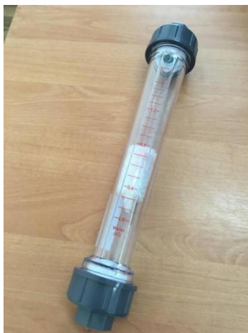
Fig.10. Rotameter, emis-meta 025A, used in the TRT equipment to measure average flow velocity.
