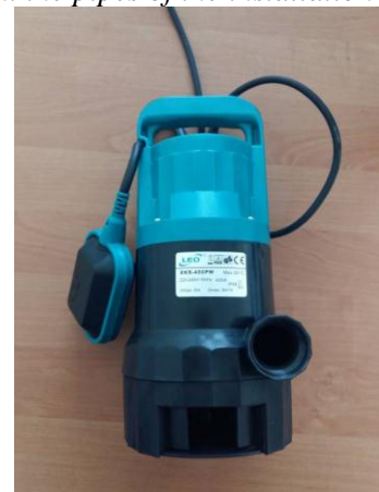
Fig. 4. Submersible pump (Leo XKS) for charging the loop with water.
