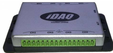
Fig. 7. Data logger used to record temperature changes during TRT process.
