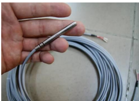
Fig. 6. Temperature sensors – Pt100, for measuring inlet and outlet temperatures of BHE
