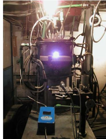
Fig. 7. The plasma chemical reactor in operation.
