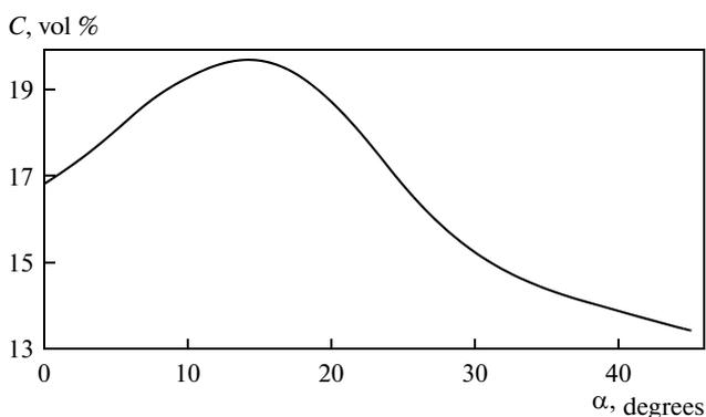
**Fig. 11.** Isosurface of pulverized coal volume concentration versus the scroll rotation angle.
