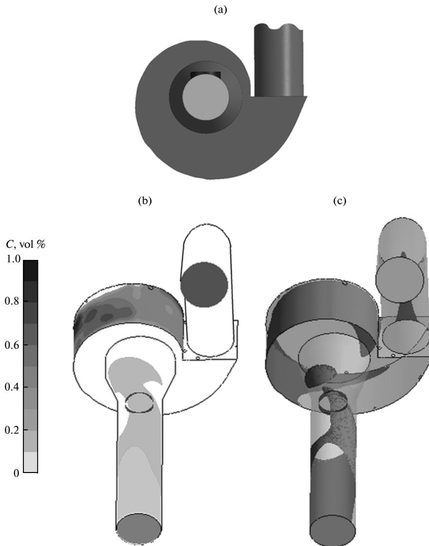
**Fig. 7.** Results from air mixture flow calculation at the scroll rotation angle equal to 0°. (a) Installation position, (b) dispersed phase volume concentration near the inner surface of the scroll and the air mixture plasma ignition, and (c) isosurface of dispersed phase volume concentration  $f = 7\%$ .
