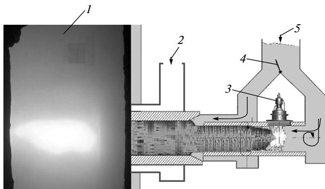
**Fig. 1.** Vortex plasma fuel system. (1) Furnace, (2) overfire air, (3) plasmatron, (4) gate, and (5) air mixture.
