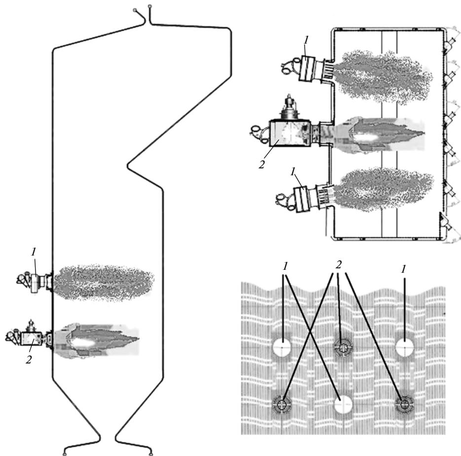
**Fig. 2.** Schematic layout of the PFS and main pulverized-coal burners in the BKZ-420 boiler at the Almaty CHP-2. (1) Standard vortex two-flow pulverized-coal burner and (2) PFS.
