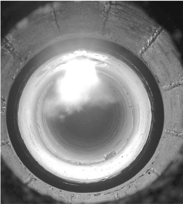
**Fig. 3.** Plasma flame in the PFS prior to supplying air mixture.
