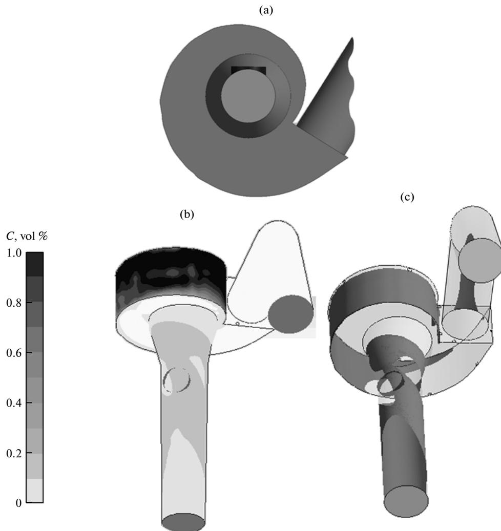
**Fig. 9.** Results from air mixture flow calculation at the scroll rotation angle equal to  $30^\circ$ . The meaning of (a) and (b) is the same as in Fig. 7, (c)  $f = 6\%$ .
