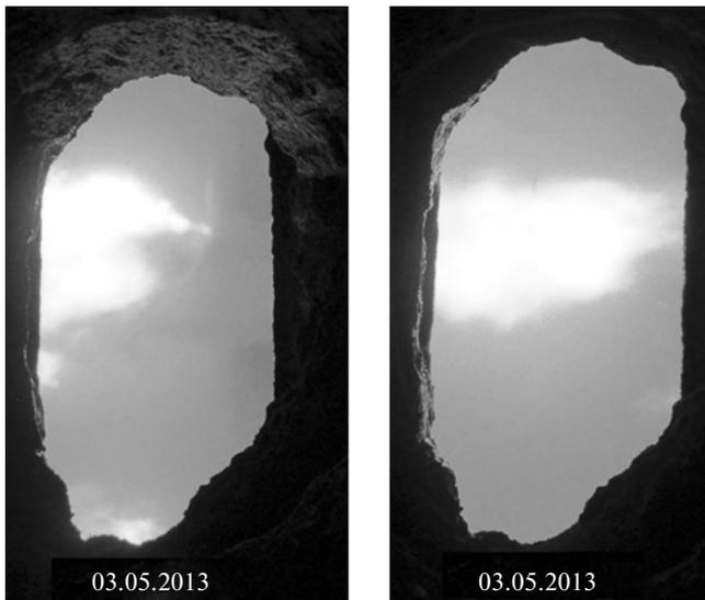
**Fig. 12.** Pulverized-coal flame from the PFS at the initial moment (a) and in 5 min after starting coal supply (b). Temperature in the flame core, °C: (a) 835 and (b) 1022.
