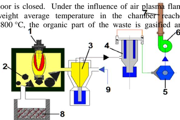
Fig. 4. Functional scheme of the experimental technological installation: 1- arc plasma torch; 2 - plasma box chamber; 3 - chamber for reburning; 4 - bag filter; 5 - ecological filter; 6 - exhaust fan; 7 - exhaust pipe; 8 - container for slag; 9 - air for reburning.
