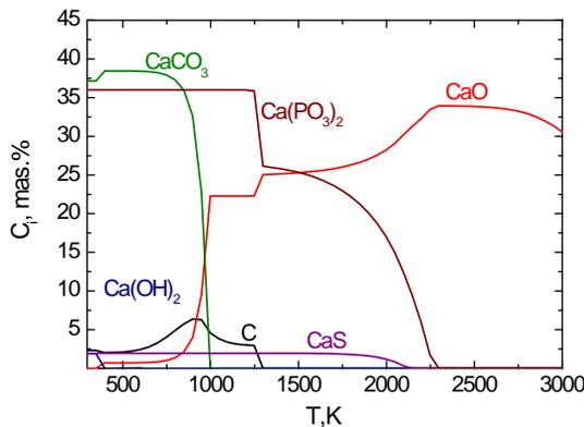
Fig. 2. Variation of the concentration of components of the condensed phase depending on the temperature of the BMW processing (Variant 1).
