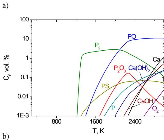
Fig. 1. Variation of the concentration of organic (a) and inorganic (b) components of the gas phase depending on the temperature of the BMW processing (Variant 1).
