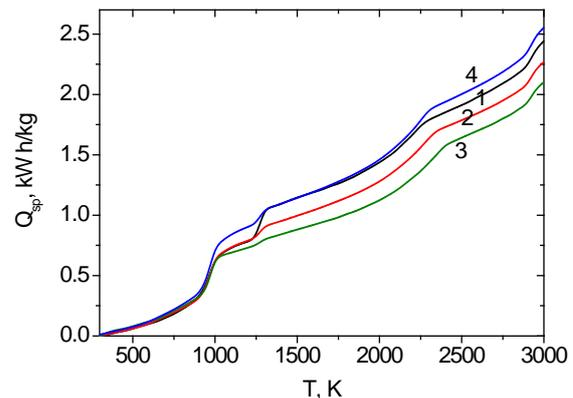
Fig. 3. Variation of specific power consumption for the BMW processing depending on the temperature: variants 1-4.
