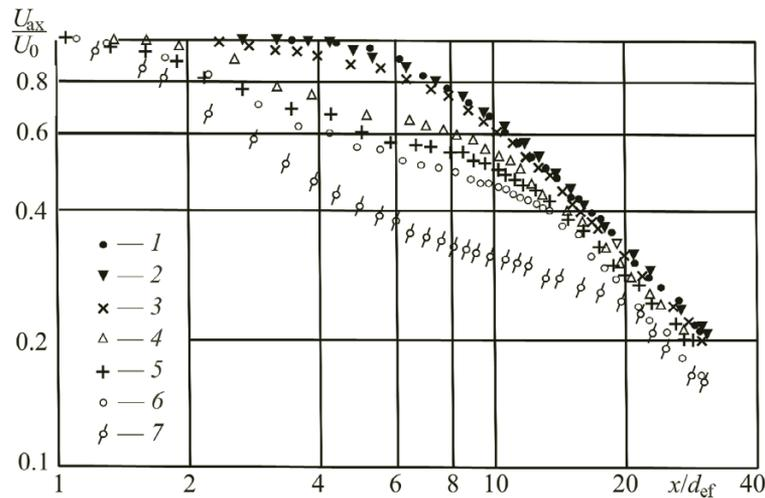
Fig. 3. Comparison of experimental data on the change in the flow velocity along the axes of the three-dimensional and axisymmetric jets at  $U_0 = 20$  m/s: 1) circular nozzle; 2)  $\lambda = 2.66$ ; 3) 5.07; 4) 7.61; 5) 11; 6) 16; 7) 25.25.
