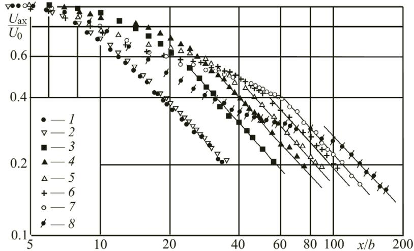
Fig. 1. Regularities in the change of the axial velocity of an axisymmetric jet issuing from a circular nozzle (1) and of three-dimensional jet issuing from rectangular nozzles with  $\lambda = 1$  (2), 2.66 (3), 5.07 (4), 7.61 (5), 11 (6), 16 (7), and 25.25 (8); solid lines, calculation by Eq. (1); points, experiment.
