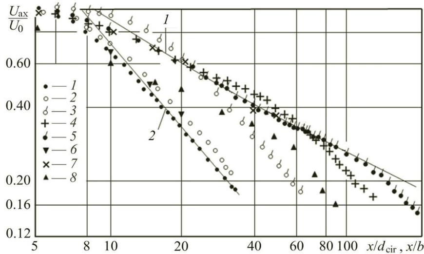
Fig. 4. Regularities in the change of the axial velocity of the three-dimensional jet at  $U_0 = 40$  m/s calculated by Eqs. (2) (top line) and (3) (bottom line): circular nozzle; 2)  $\lambda = 1$ ; 3) 2.66; 4) 11; 5) 25.25; 6) 1 [10]; 7) 10 [10]; 8) 12.4 (slit orifice [4]).
