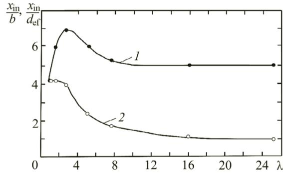
Fig. 2. Length of the initial portion of the jet vs. the nozzle aspect ratio at  $U_0 = 20$  m/s: 1)  $x_{in}/b$ ; 2)  $x_{in}/d_{ef}$ .
