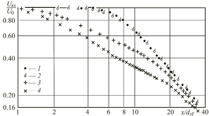
Fig. 5. Comparison of experimental data on attenuation of the axial velocity of the three-dimensional and axisymmetric jets at  $U_0 = 40$  m/s: 1) circular nozzle; 2)  $\lambda = 2.66$ ; 3) 11; 4) 25.25.
