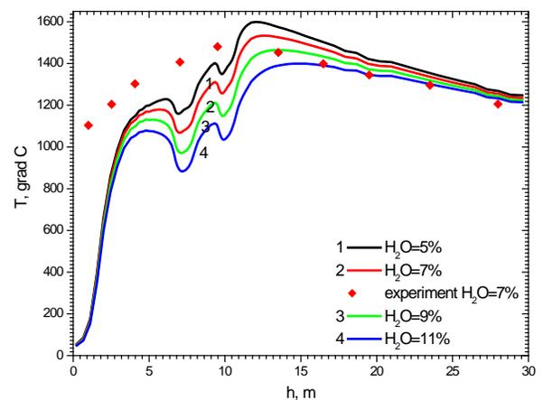
Fig. 2 Temperature distribution along the chamber height for coal burning with different water content.
