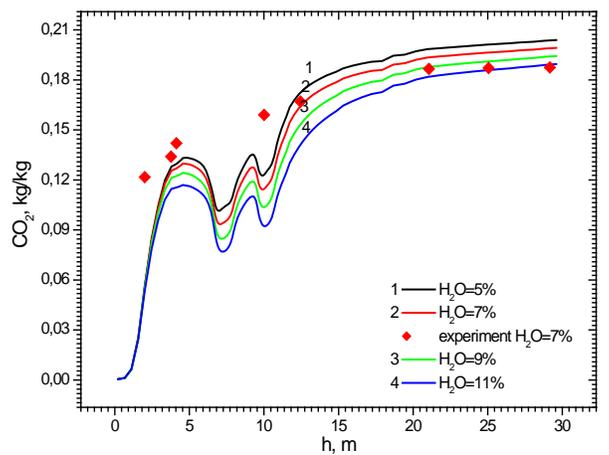
Fig. 9  $CO_2$  concentration distribution along the chamber height for coal burning with different water content.
