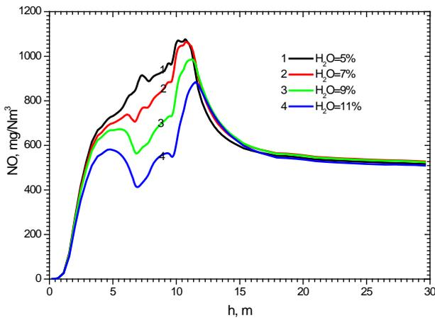
Fig. 10 NO concentration distribution along the chamber height for coal burning with different water content.
