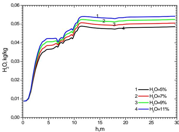
Fig. 6 Water concentration distribution along the chamber height for coal burning with different water content.
