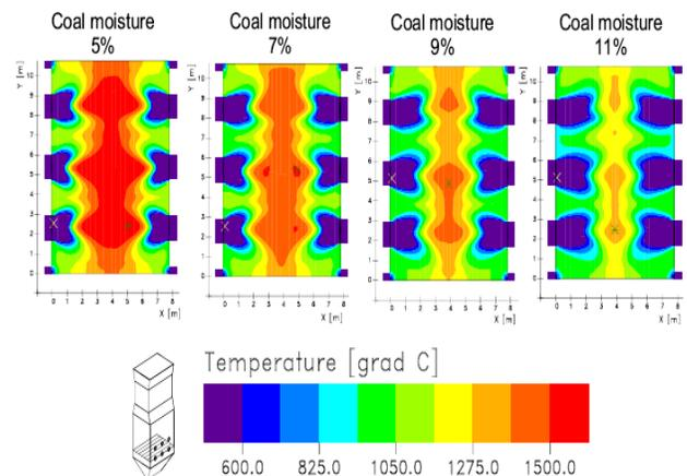
Fig. 3 Temperature distribution in cross section of the furnace in the lower level of the burners for coal burning with different water content.
