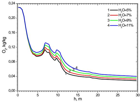
Fig. 4  $O_2$  concentration distribution along the chamber height for coal burning with different water content.
