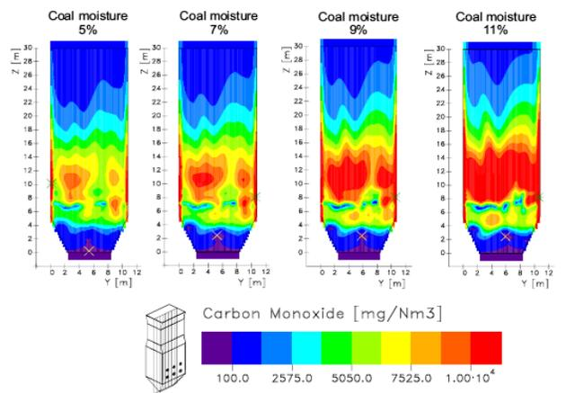
Fig. 8 CO distribution in the central section of the furnace for coal burning with different water content.
