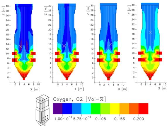
Fig. 5 Oxygen concentration distribution in the central section of the furnace for coal burning with different water content.
