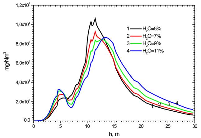
Fig. 7 CO concentration distribution along the chamber height for coal burning with different water content.
