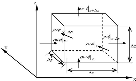
Fig 1. Control volume for the generalized transport equation
