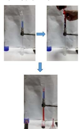
Fig. 6 Study of the efficiency of separation of chloroform and water by a hydrophobic oleophilic membrane based on a stainless steel mesh of grade 400, coated with PTFE
