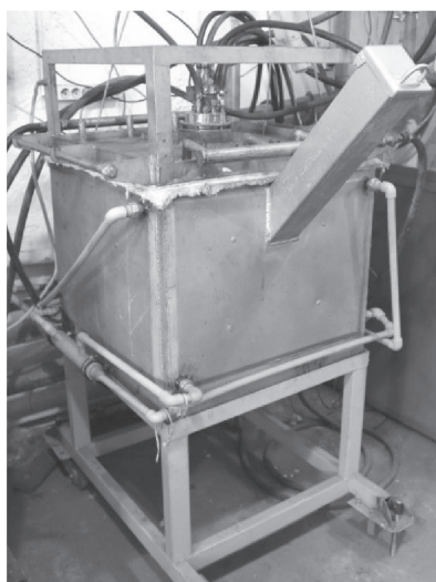
Fig. 2. Experimental setup for RSW plasma processing on the test bench of the Scientific and Technical Organization "Plazmotekhnika."
