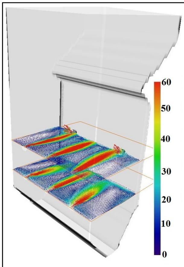
**Fig.3.** Full velocity vector fields in the combustor cross section at a conventional coal combustion
