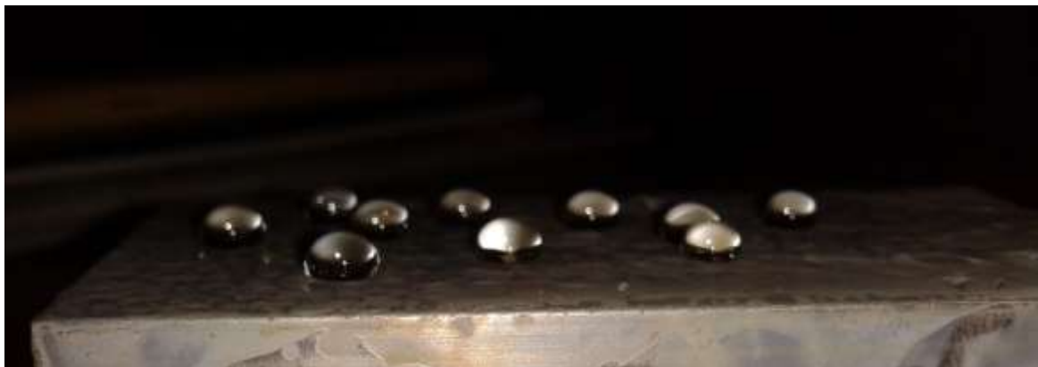
Fig. 3. Behavior of water droplets on a synthetic de-icing coating applied to a metal surface.
