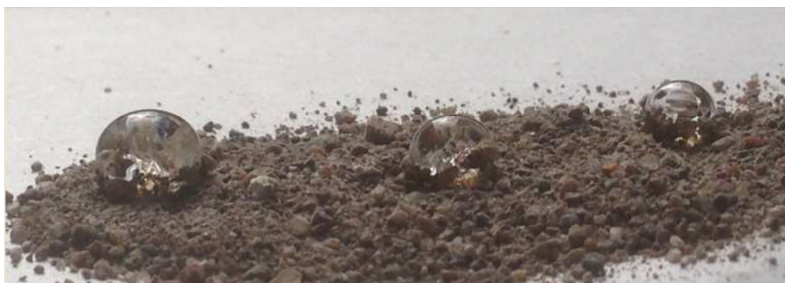
Fig. 7. Water droplets on the surface of hydrophobic sand
