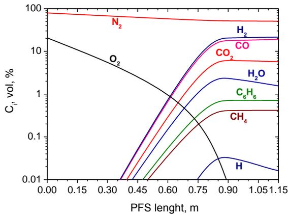
Figure 3. Gas phase components concentrations along the PFS.
