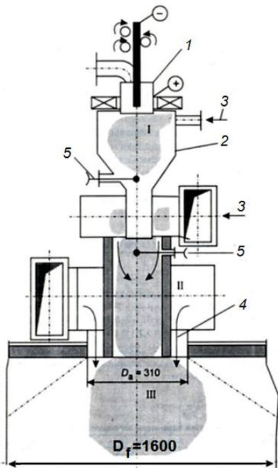
Figure 1. Layout drawing of plasma-fuel system and experimental furnace: 1 - plasmatron; 2 - chamber of electro-thermochemical preparation of fuel; 3 - pulverised coal; 4 - secondary air; 5 - slot for measuring; I - zone of air/coal mixture interaction with plasma flame and HRF forming; II - zone of HRF interaction with the main air/coal mixture; III - zone of the fuel self-ignition.
