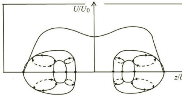
Fig. 6. Simplified scheme of an instantaneous pattern of large-scale vortices in the transient region of a three-dimensional jet and influence of these vortices on the flow-velocity distribution in the jet at  $\lambda = 11$ ,  $U_0 = 6$  m/s, and  $x/b = 12$ .
