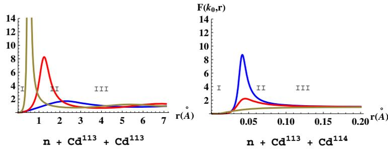
**Fig. 1** Neutron resonances on a two nucleus subsystem: left “ $n + A + A$ ”-system, where the resonance energy and the width of the  $(n + A)$ -subsystem are  $E_R = 2.77$  meV,  $\Gamma = 0.5$  meV,  $A \equiv \text{Cd}^{113}$ ; on the right “ $n + A + B$ ”-system, where the resonance energy and the width of the  $(n + B)$ -subsystem are  $E_R = 56.4$  eV,  $\Gamma = 0.08$  eV,  $B \equiv \text{Cd}^{114}$
