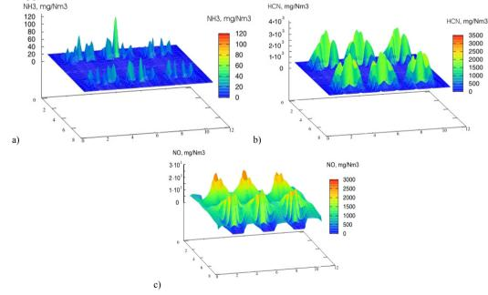
Fig. 2. Distribution of the concentration (a) - ammonia NH<sub>3</sub>; (b) - HCN; (c) - NO nitrogen monoxide in the combustion chamber of the boiler SB-39 in the field of lower level of the burners
