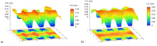
Fig. 1. 3D concentration distribution of  $CO_2$  in the combustion chamber of the SB-39 in the field of burner (a) - lower level; (b) - the top-level
