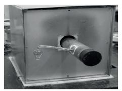
Fig. 3. Nichrome furnace with quartz reactor.
