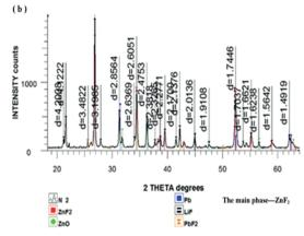
Fig. 9. X-ray analyses of PRPS with magnesium (a) and with zinc (b).
