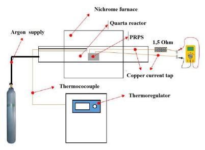
Fig. 2. Principal scheme of experimental setup.
