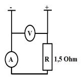
Fig. 5. Scheme of current and voltage measurement in the PRPS system.
