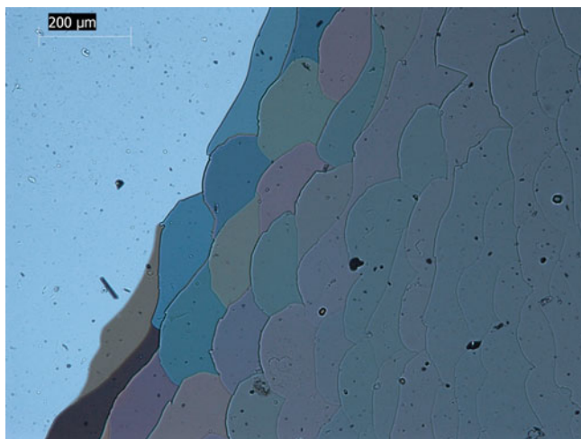
Fig. 113.5 The surface of the diamond -like carbon film obtained with an optical microscope
