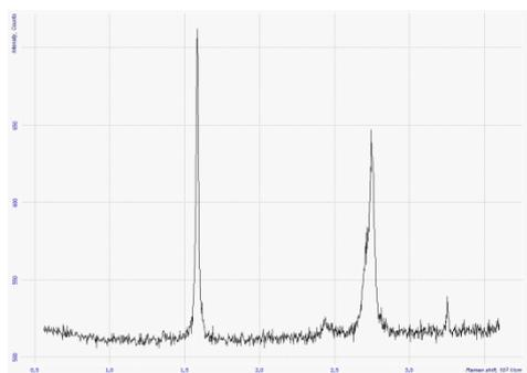
**Figure 2** Raman spectrum of graphite with benzene after processing with ultrasound
