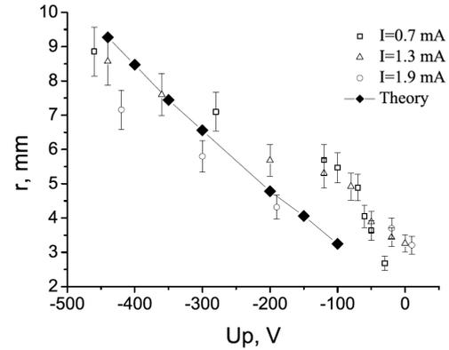
**Fig. 4** Comparison of experimental data with theoretical results for different values of the discharge current. The pressure in the discharge tube  $P=0.3$  torr.
