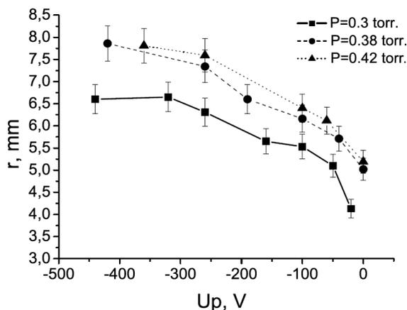
**Fig. 2** Dependence of the dust-free region's radius on the probe potential  $U_p$  at the different values of gas pressure.
