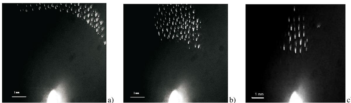
**Fig. 1** Dust free region in the dependence on the voltage on the probe. a)  $U_p = -260$  V ; b)  $U_p = -100$  V; c)  $U_p = -60$  V;
