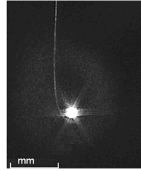
Fig. 5: Trajectory of the dust particle in the probe sheath. Example 2.
