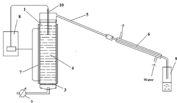
Fig. 4. Scheme of apparatus for the thermal processing of oil sands: 1 – cylindrical reactor, 2 – tube, 3 – Perforated diaphragm, 4 – raw material, 5 – connecting pipe for output gas and products, 6 – refrigerator, 7 – electric furnace, 8 – thermoregulator, 9 – receptacle.
