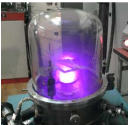
Figure 2. Magnetron discharge in the atmosphere of aromatic hydrocarbons.
