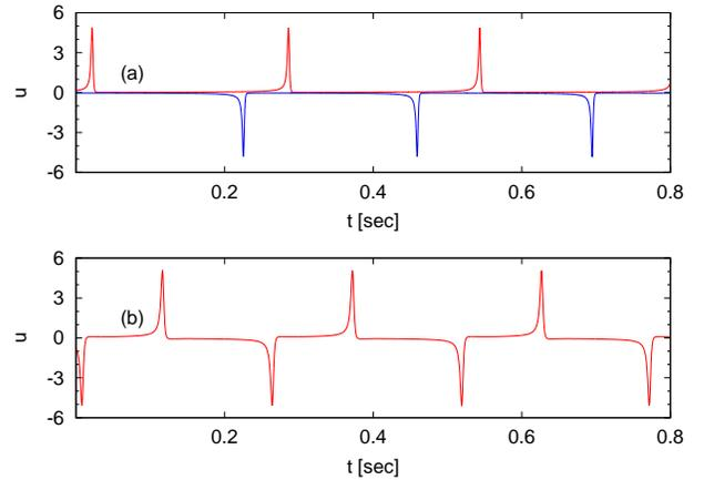
Fig. 4. Temporal evolution close to the gluing bifurcation. (a): oscillations on limit cycles with 1 loop prior to the bifurcation; (b): oscillations on the limit cycle with 2 loops.
