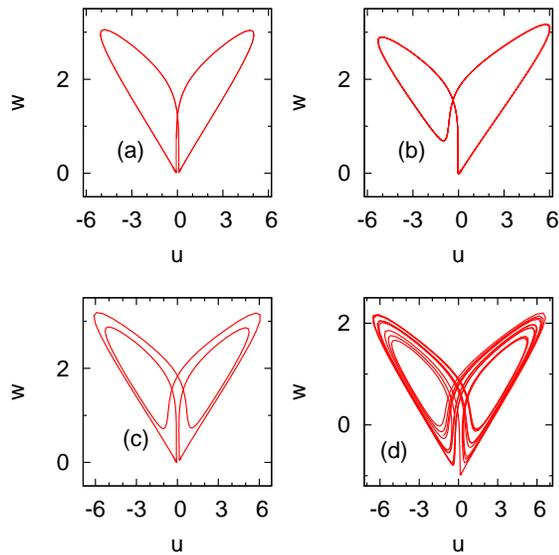
Fig. 5. Further evolution of the attracting set. (a): stable symmetric orbit with two turns; (b): asymmetric orbit with two turns; (c): symmetric orbit with 4 turns born from the secondary gluing bifurcation; (d): chaotic attractor.
