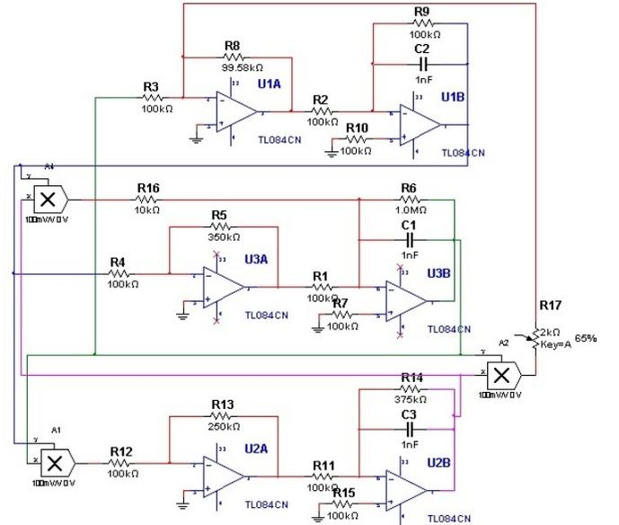
Fig. 1. Electronic circuit for modeling Eqs (2). The values of the resistors and capacitors are shown on the scheme. The analog multipliers (denoted by crosses) are of the type AD633AN.
