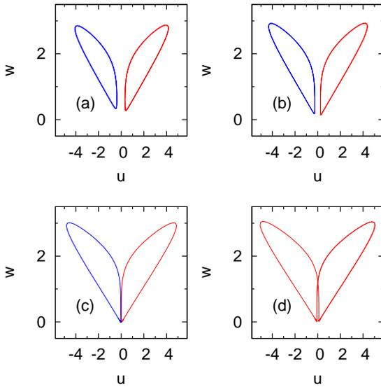
Fig. 2. Principal gluing bifurcation: Evolution of the attracting set. (a,b): two stable periodic orbits. (c): formation of two trajectories, homoclinic to the equilibrium. (d): stable self-symmetric orbit with two loops.
