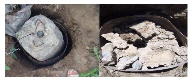
a) b) a) Monolithic concrete block, b) Monolithic concrete block is crushed by gas generator.
