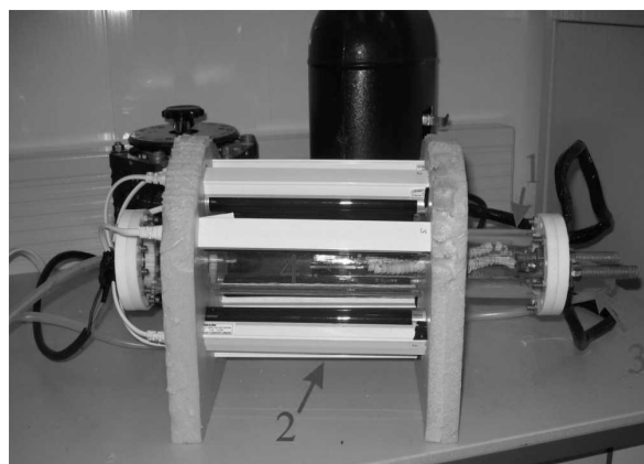
1 – Quartz tube (reaction chamber); 2 – source of ultraviolet irradiation; 3 – clamp terminals, 4– sample (substrate holder)
