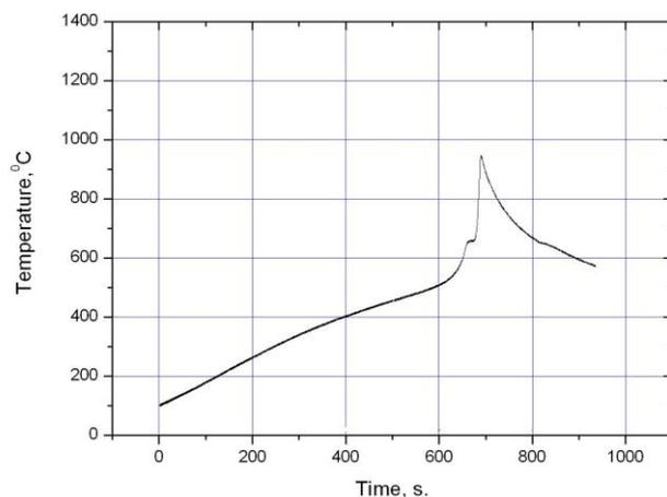
**Figure 5. A thermogram of thermal explosion of Mg+2.1B mixture exposed to 2 min preliminary mechanical processing.**
