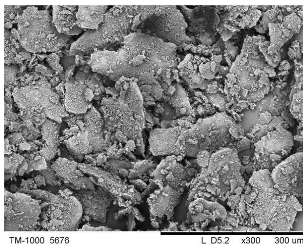
**Figure 1. Microphotography of Mg+2.1B mixture after 30 s mechanical processing.**
