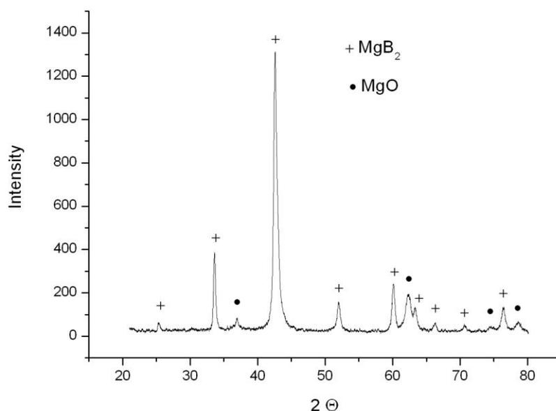
**Figure 7. X-ray phase diagram of the Mg+2.1B mixture thermal explosion (6 min preliminary mechanical processing).**
