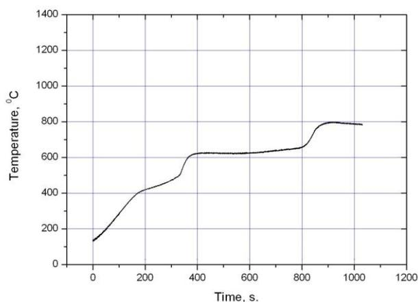
**Figure 3.A typical thermogram of thermal explosion of Mg+2.1B mixture (30 sec preliminary mechanical processing).**
