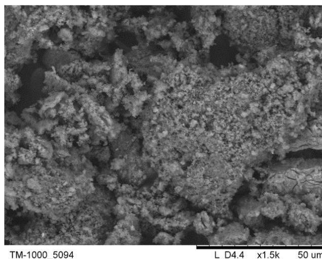
**Figure 8. Microphotography of Mg+2.1B mixture thermal explosion products (6 min preliminary mechanical processing).**
