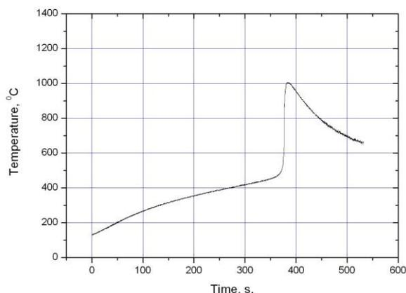
**Figure 6. Thermogram of thermal explosion of Mg+2.1B mixture exposed to 5 min preliminary mechanical processing.**
