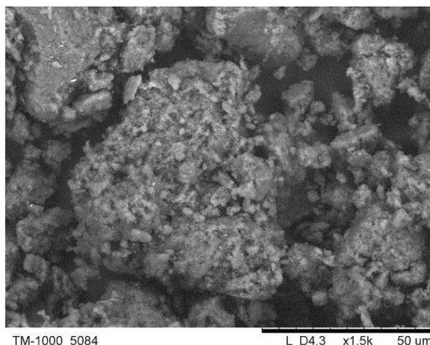
**Figure 2. Microphotography of Mg+2.1B mixture after 5 min mechanical processing.**
