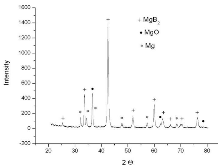
**Figure 4. X-ray phase diagram of the Mg+2.1B mixture thermal explosion (30 sec preliminary mechanical processing).**
