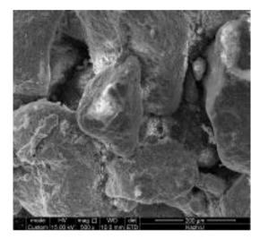
Figure 5. Electron micrograph of the surface of the grains of sand.
