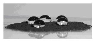
Figure 2. Drops of water on the surface hydrophobic sand.
