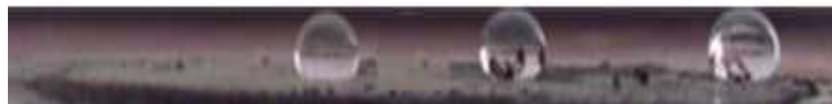
Fig. 3. The behaviour of water droplets on a silicon substrate with the deposited hydrophobic soot on it.
