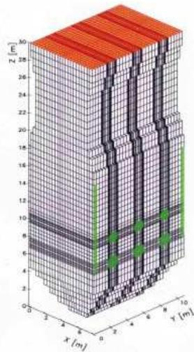
**Figure 1 General view of the division into the cells of combustion chamber of the boiler SB-39 on Aksu TPP.**
