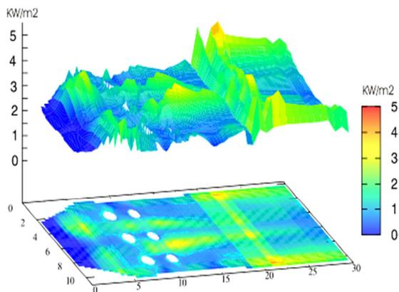
**Figure 3** Three-dimensional distribution of the convective heat flux on the front wall of the combustion chamber of the boiler SB-39.
