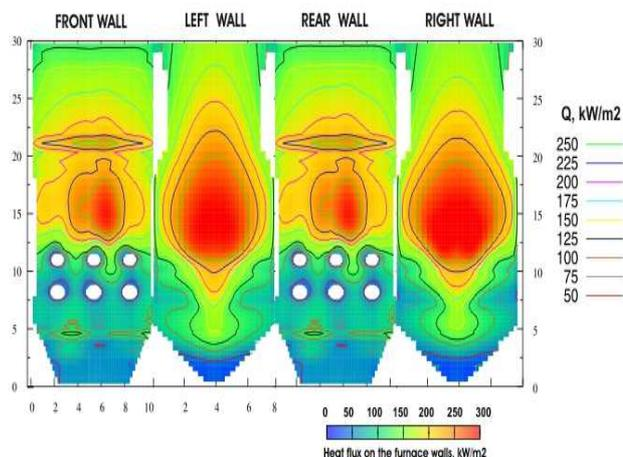
**Figure 5** Distribution of the total heat flux on the walls of the combustion chamber of the boiler PK-39.
