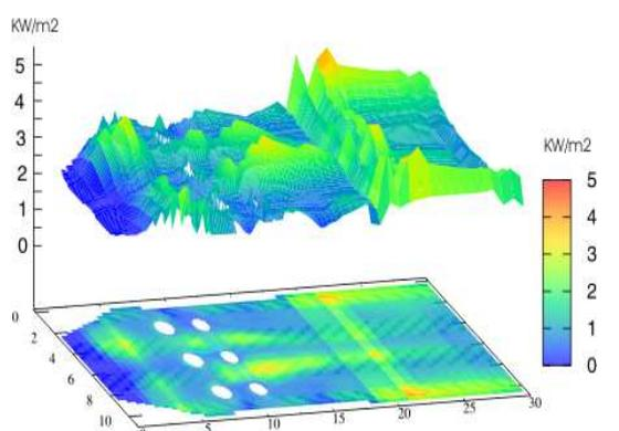
**Figure 4** Three-dimensional distribution of the convective heat flux on the back wall of the combustion chamber of the boiler SB-39.
