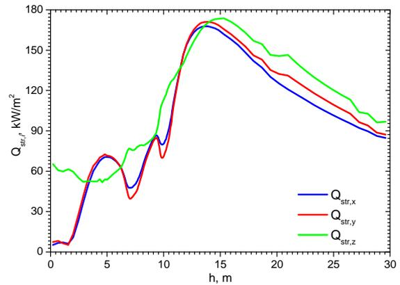
**Figure 2 Distribution of average height values of heat flux due to radiation in the coordinate directions *x*, *y*, *z*.**
