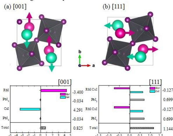
Figure 2. Berry phase polarization calculation from undistorted tetragonal phase to a fully distorted orthorhombic phase of (a) [001] projection of CsRbPb<sub>2</sub>I<sub>6</sub> and (b) [111] projection of CsRbPb<sub>2</sub>I<sub>6</sub>.
