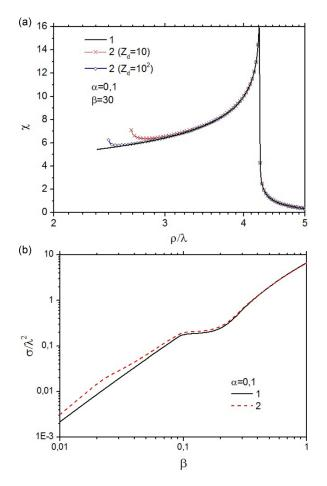
FIG. 3. In (a), the scattering angle obtained using the Yukawa potential (line 1) and the interaction potential (5) of the ion with the spherical dust grain (line 2). In Figure 3(b), the scattering cross section obtained using the Yukawa potential (line 1) and the interaction potential (5) of the ion with the spherical dust grain (line 2) is shown.
