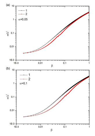
FIG. 7. The scattering cross section obtained using the Yukawa potential (line 1) and the interaction potential (13) (line 2) taking into account an induced dipole moment.
