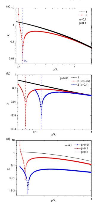
FIG. 5. In (a) and (b), the dust particle-dust particle scattering angle obtained using the Yukawa potential (line 1) and the dust particle-dust particle interaction potential (13) (line 2), which takes into account an induced dipole moment, is shown. In Figure 4(c), the scattering angle obtained using the dust particle-dust particle interaction potential (13) for the different values of  $\beta$  is given.
