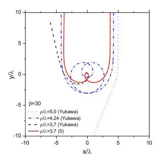
FIG. 4. Ions trajectories during collisions at  $\alpha = 1$ , Z = 10. The scattering center is located at x = 0, y = 0.
